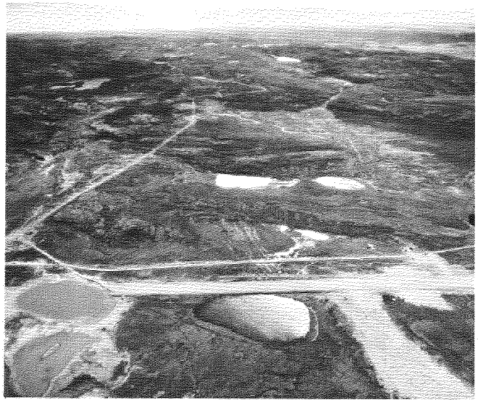
Fig. 4. Airstrip of station in Fig. 3. Note material pulled in from moraine. Road follows bare rock surface
